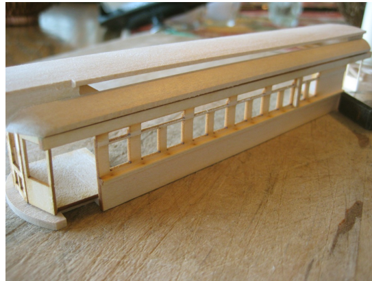
Side panel placed against ends and roof and aligned to door openings. Check for correct roof over hang and front floor sill.
