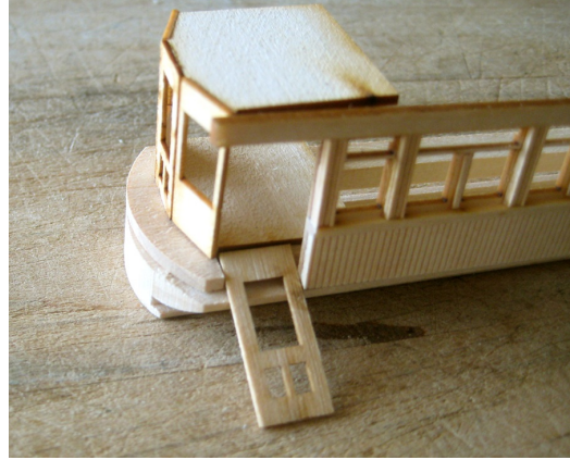
Showing the placement of the walk through door. Note the location of the sill and round of the roof assembly. Side panel is located from this end and all trimming of the side should be done at the freight door end. A similar layout should be done with the Sacramento Northern coach and other passenger applications to establish the location of the sills in relation to the roof
