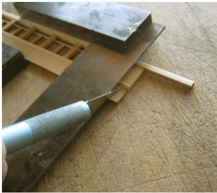
Showing the trimming of the side panel with a machinist's square.
